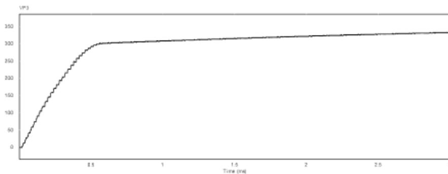
Figure 14. Output Voltage of the converter is 299.8V for input voltage of 25 V with controller
