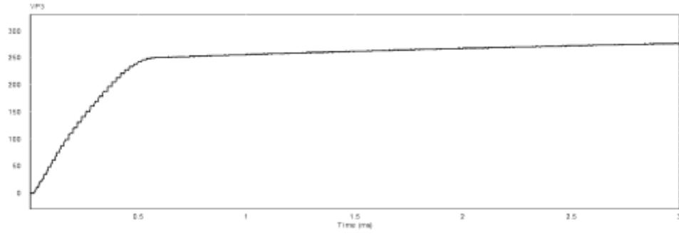
Figure 11. Output Voltage of the converter is 250 V for input voltage of 25 V without controller
