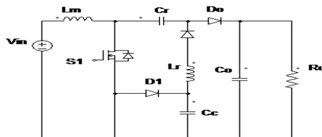
Figure 2. Single Switched Inductor Capacitor Coupled Converter
