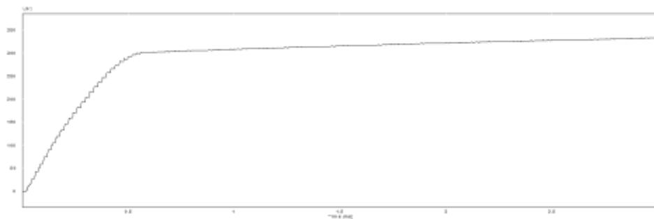
Figure 10. Output Voltage of the converter is 300V for input voltage of 30 V without controller
