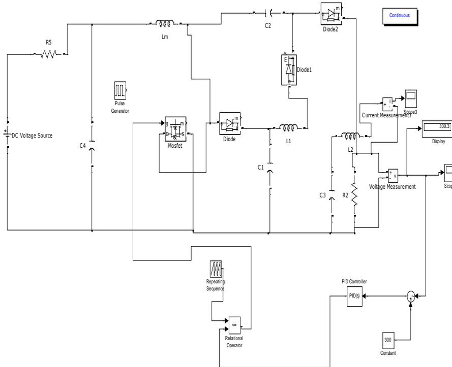
Figure 9. Simulation Diagram of the complete System
