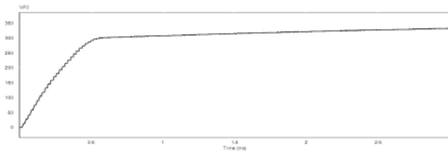
Figure 13. Output Voltage of the converter is 299.8V for input voltage of 30 V with controller
