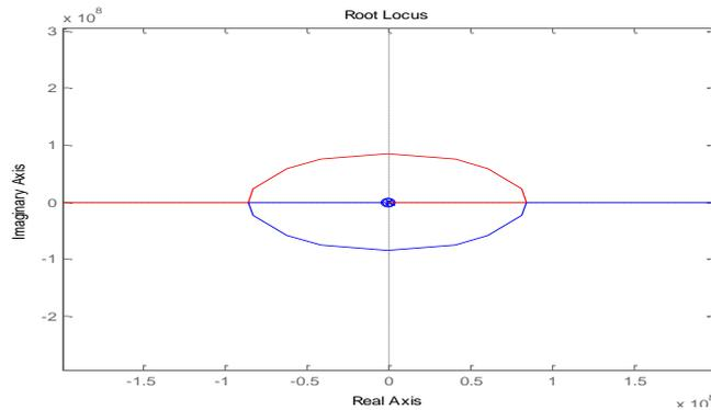
Figure 8. Root Locus Plot of the converter without controller
