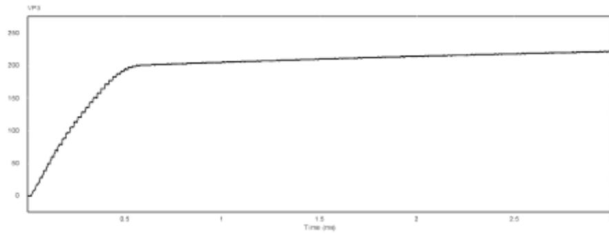
Figure 12. Output Voltage of the converter is 200V for input voltage of 20 V without controller
