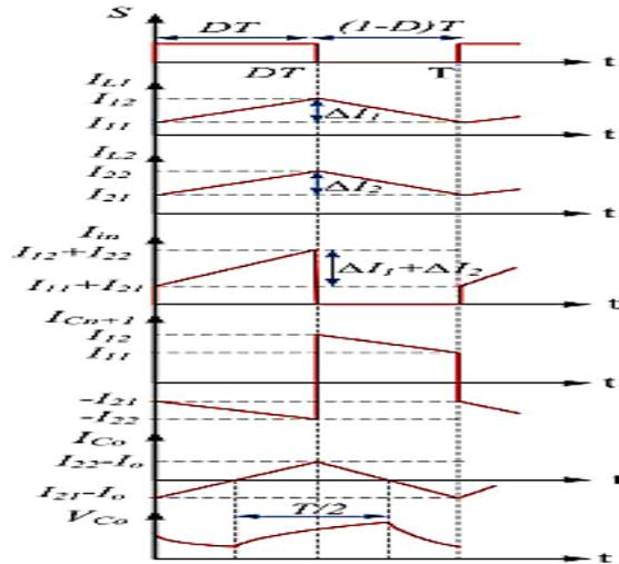
Figure 4. Waveforms of proposed enhanced zeta
