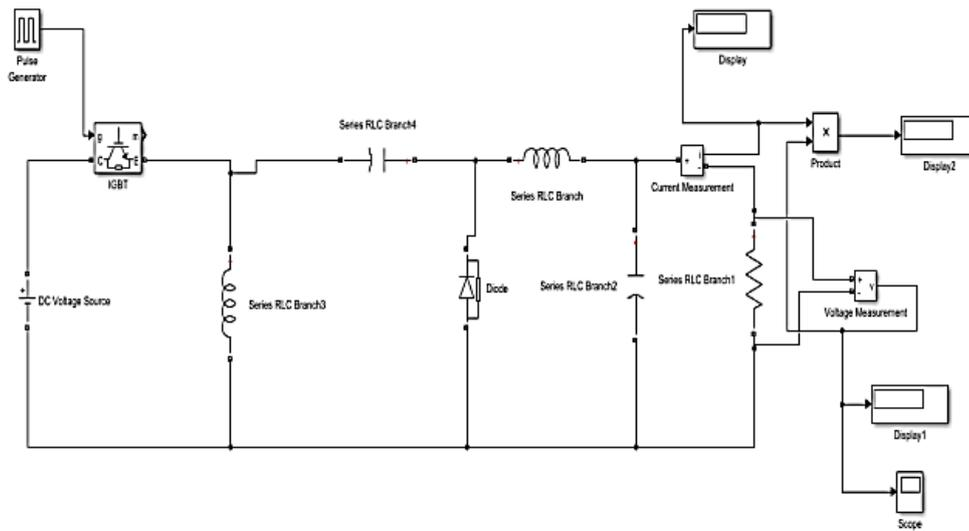
Figure 5. Simulation diagram of existing zeta converter
