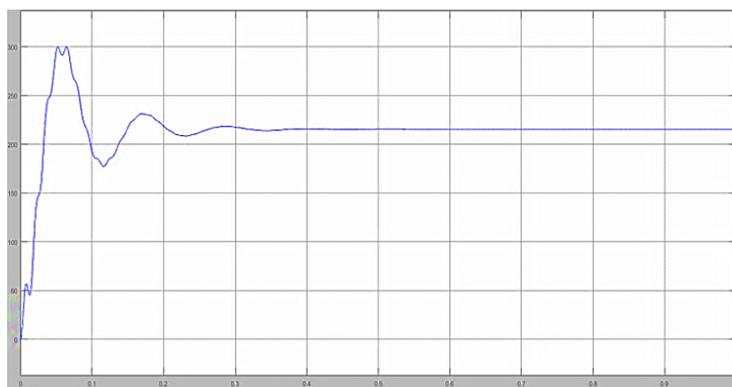
Figure 6. Existing zeta converter in boost mode (voltage output)
