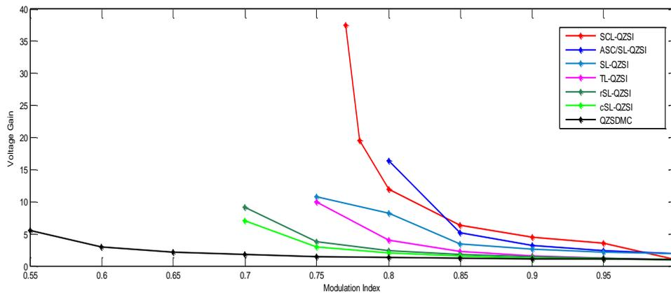
Figure 12. Plot of Modulation Index (M) vs Voltage Gain (G)
