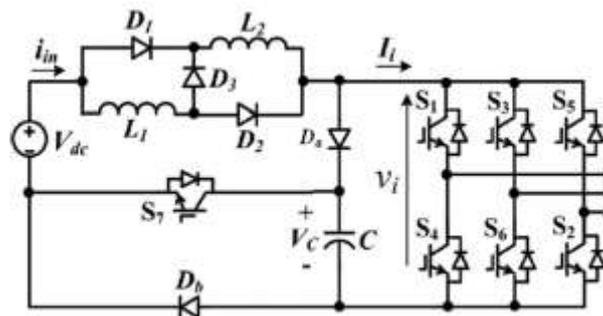
Figure 10. Active Switched Capacitor/ Switched Inductor QZSI
