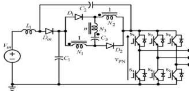
Figure 6. Switched- Coupled Inductor Quasi Z- Source Inverter
