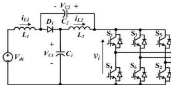
Figure 2. Basic Quasi Z-Source inverter
