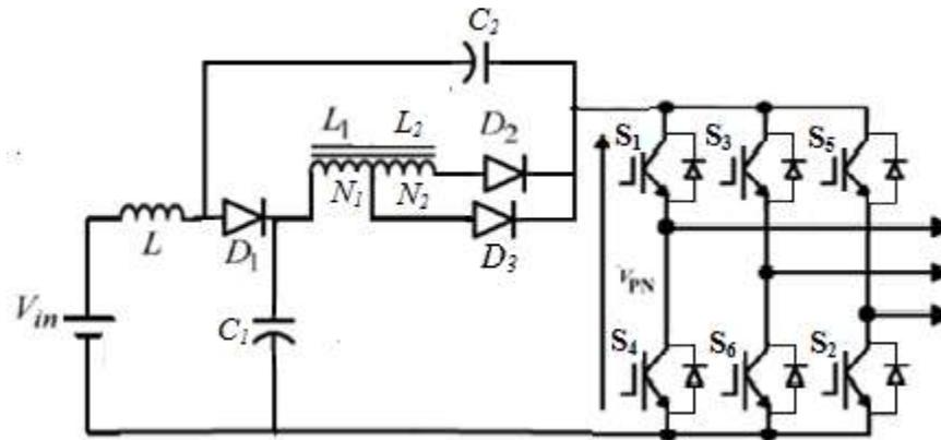
Figure 7. Tapped inductor Quasi Z-Source inverter
