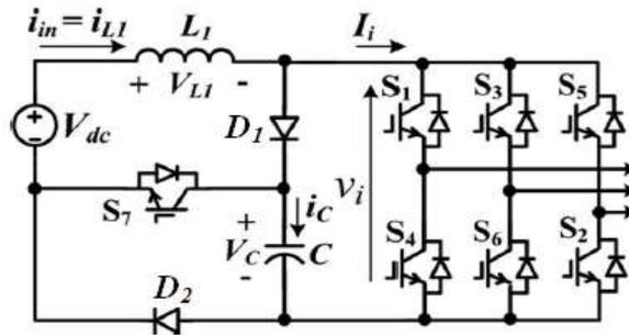
Figure 9. Basic Active Switched Capacitor QZSI
