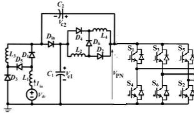
Figure 5. capacitor Switched-Inductor QZSI
