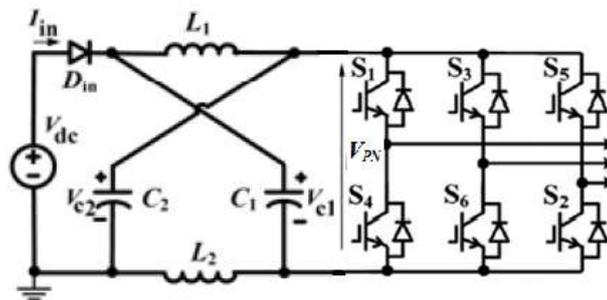
Figure 1. Basic Z-Source Inverter
