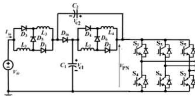
Figure 4. ripple Switched-Inductor QZSI
