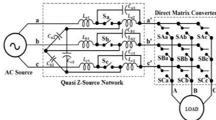
Figure 8. Quasi Z-Source Direct Matrix Converter
