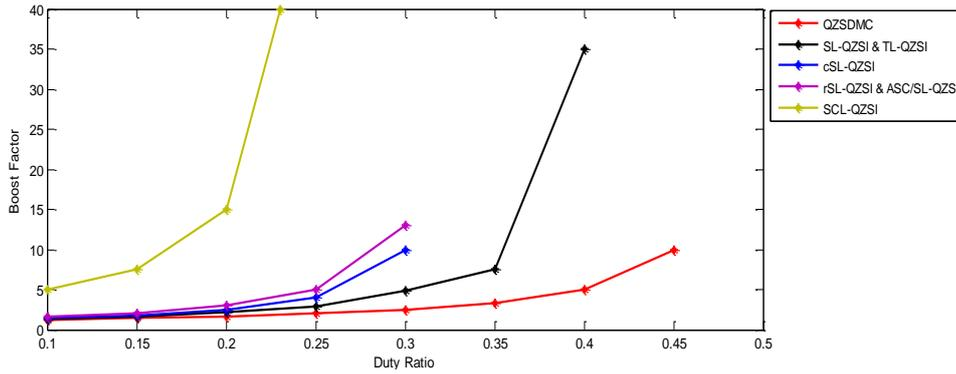
Figure 11. Plot of Duty Ratio (D) vs Boost factor (B)
