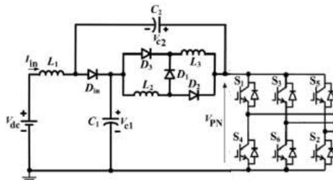
Figure 3. Switched-Inductor quasi Z-Source Inverter
