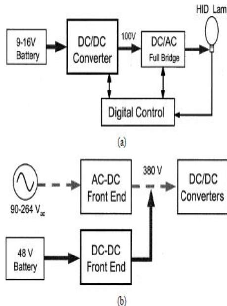
Figure 2. Applications of the dc-dc converter a) HID lamp ballast b) dual-input front –end converters.
