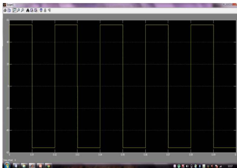
Figure 9. Output Voltage waveform for Single Phase Full Bridge Inverter
