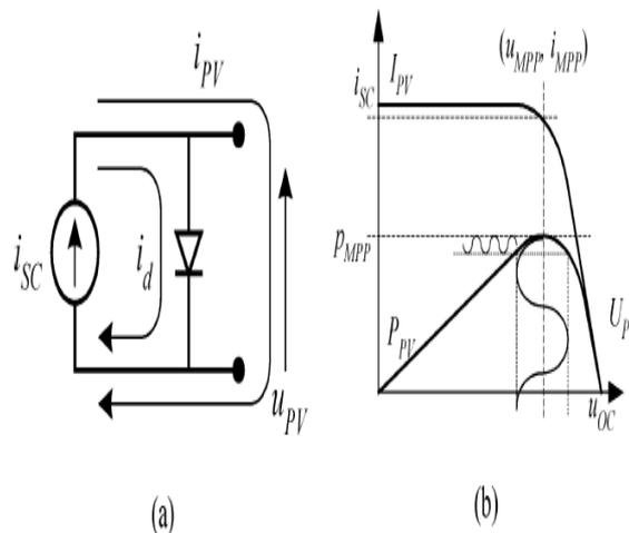
Figure 4. Model and Characteristics of PV Panel
