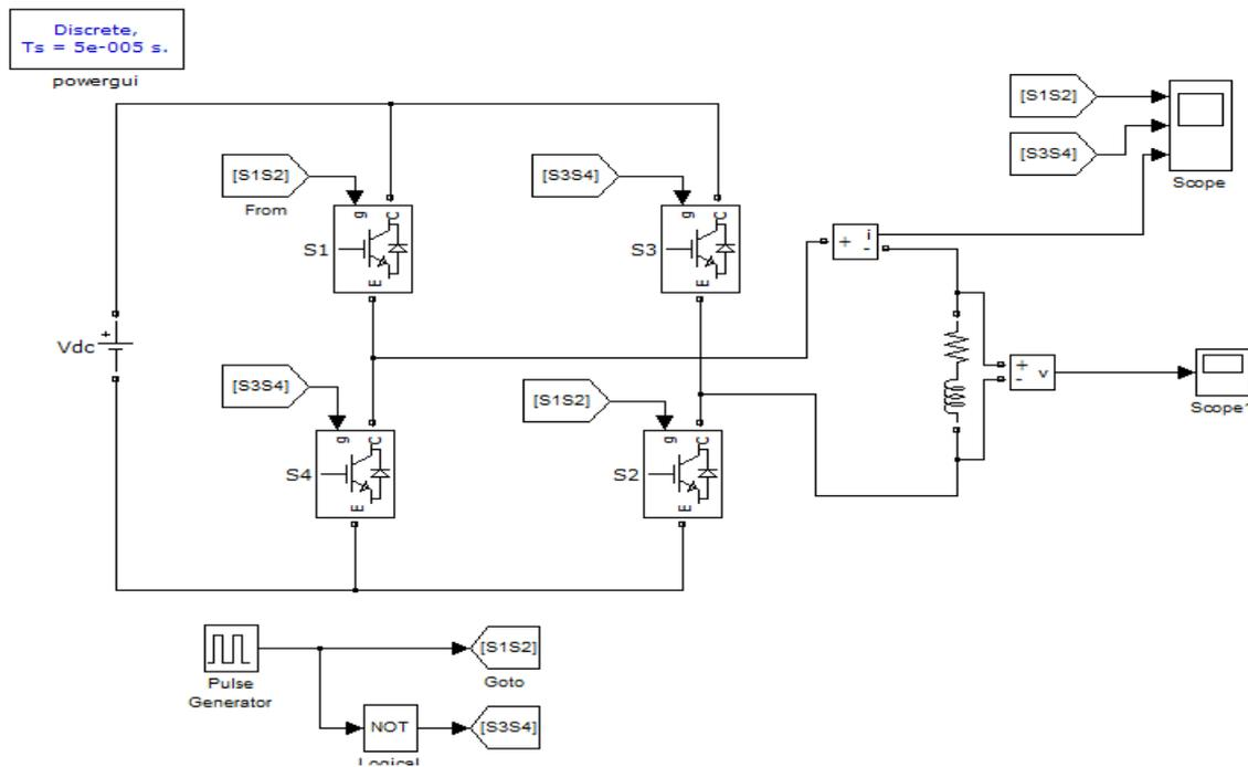
Figure 7. Simulation of Single Phase Full Bridge Inverter using Matlab/Simulink
