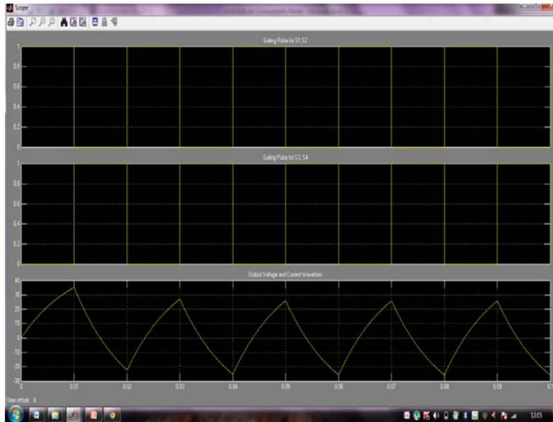
Figure 8. Pulse voltage and Output Current waveform for Single Phase Full Bridge Inverter
