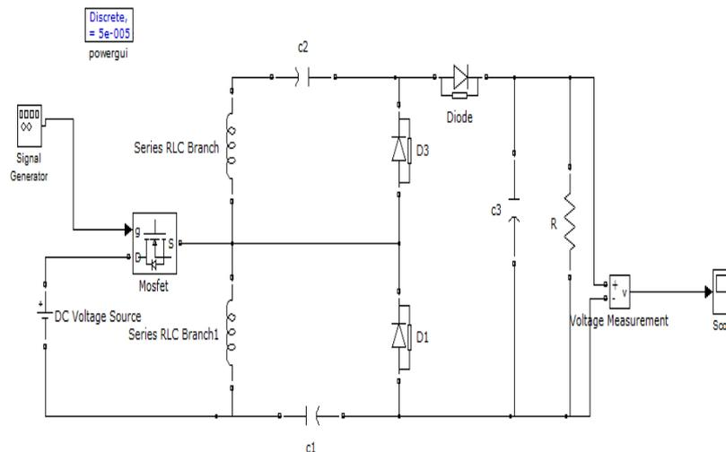
Figure 5. Simulation of Boost Converter using Matlab/Simulink
