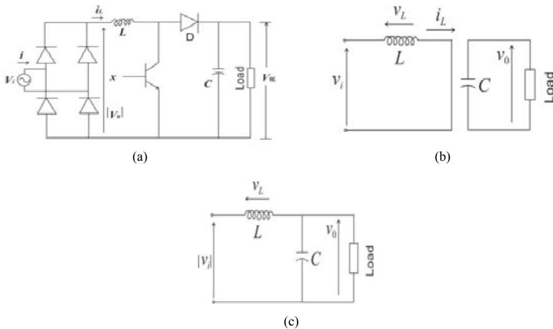
Figure 2. Single-Phase Boost Rectifier for the Electric Drive System: (A) Power Circuit and Equivalent Circuit for Transistor T in (B) On-State and (C) Off-State
