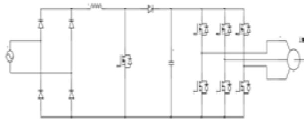
Figure 1. 1-φ Boost Rectifier with he 3-φ Electric Drive System
