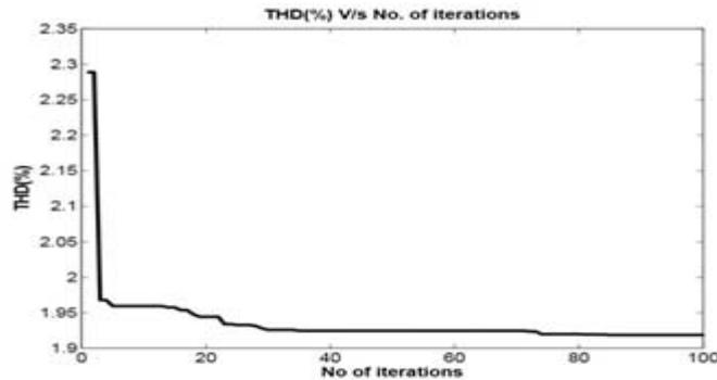
Figure 3. Particle Swarm Optimization THD vs No. of Iterations
