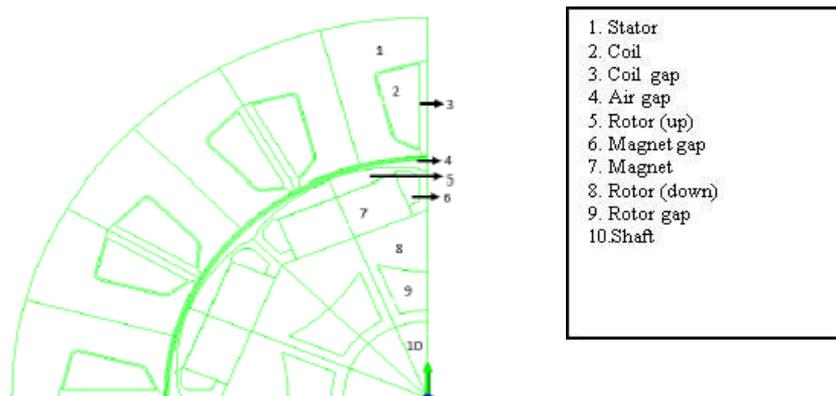
Figure 1. Geometry designed of electric generator
