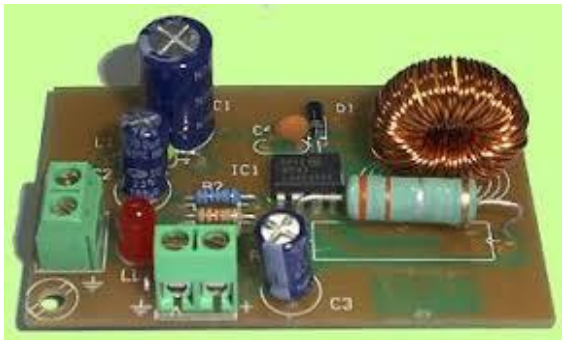
Gambar 2.3 Rangkaian converter step up dc to dc
