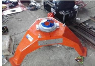
Gambar 2.8 Spider Seafloor Platforms
