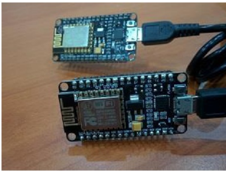
Figure 4.4. Sensor node Using NodeMCU along with the Sensor
