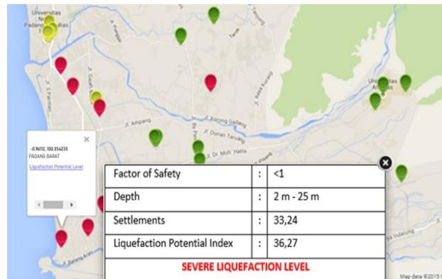
Fig. 9. Liquefaction Potential Information at a coordinate in the map.
