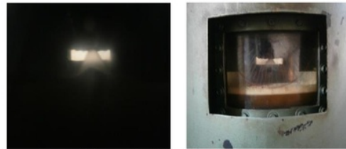
Figure 8 Spray Angle of Sample I and Sample IV
