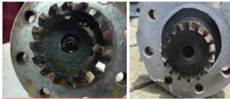
Figure 15 Deposit at No 1 Nozzle, after used Sample I (left side) and Sample III (right side)
