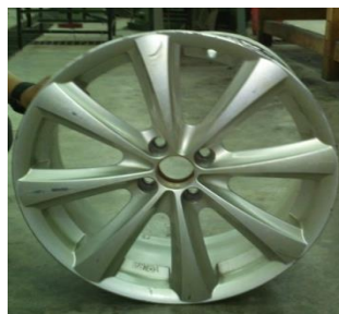
Gambar 2. Velg mobil Toyota Corolla Altis jenis paduan aluminium A413.0
