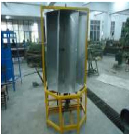
Gambar 3.7 Prototipe turbin angin savonius
