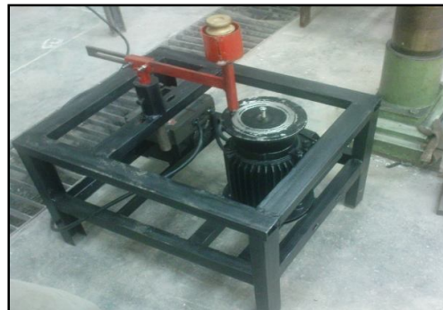
Gambar 1. Alat Uji keausan Standar ASTM G99-04 tipe pin on disk
