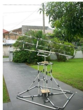
Gambar 6 Antena *Stacking* Yagi
