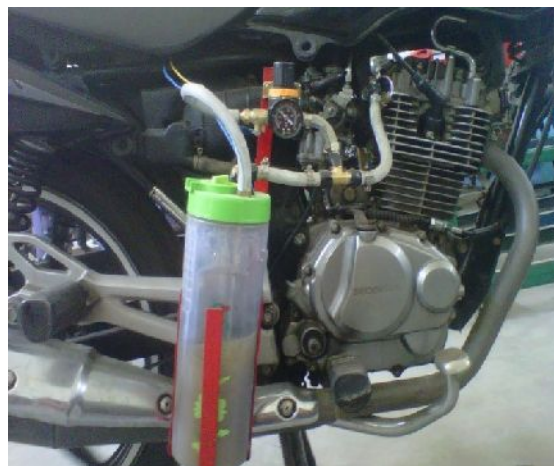
Gambar 5. Instalasi Sistem Water Injection
