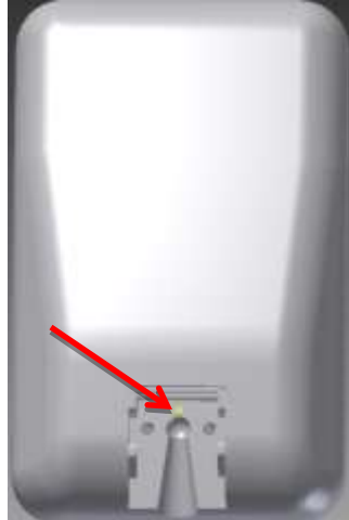
Gambar 1. Letak Gate Location
