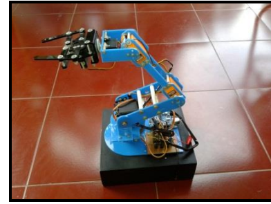
Gambar 18. Simulator arm robot 5 dof
