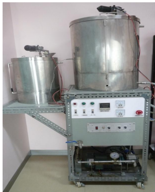
Fig. 4 Continuous ultrasonic biodiesel reactor designed by Untoro and Dimiyati, suitable for small scale and medium biodiesel plant.
