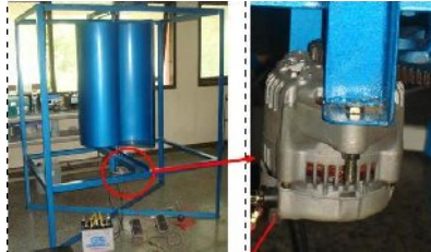
Gambar 8. (a) Hasil rancang bangun turbin angin model Savonius 2 sudu (b) Generator AC ( alternator )
