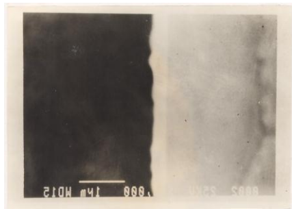
Figure 2a. Photograph of Pb thin film produced, after 4200 laser shots irradiation. The thickness of the film was 0.5 \mu\text{m} .
