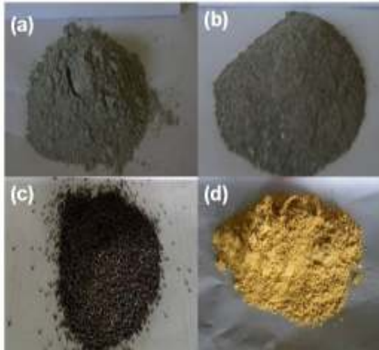
Gambar 2. Material penguat (filter) a. Bubuk basalt, b. Bubuk cangkang kerang, c. Aluminium Oxide, d. Phenolic Resin
