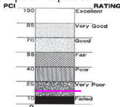
Gambar 9. Diagram nilai PCI segmen 63 (Shahin, M.Y. 1994)
