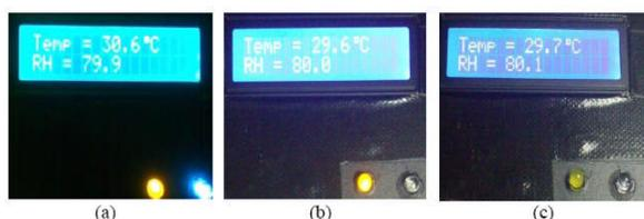
Gambar 11 Kondisi LED biru saat *set point* kelembaban 80% : (a) kelembaban < *set point*, (b) kelembaban = *set point*, (c) kelembaban > *set point*
