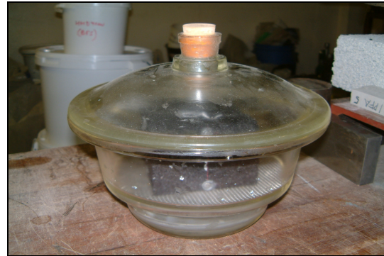
Figure 8. Sample conditioning in desiccators, with hygrostatic solution at the base.
