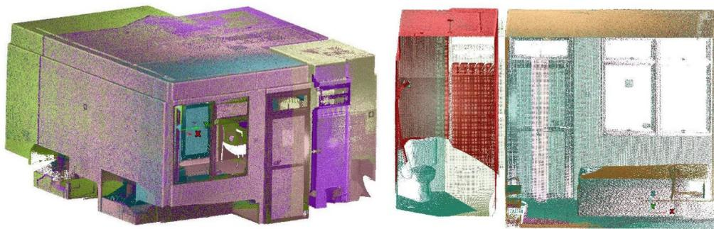
Figure 5. 'Point clouds' processing of outside and inside room with 12.5 mm density
