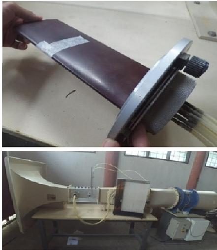
**Gambar 1.** Airfoil Naca 23012 & wind tunnel subsonic
