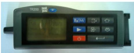
**Gambar 4.** *Roughness Tester* TR200
