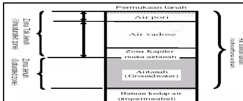
Gambar 1. Distribusi Vertikal Airtanah (Todd, 1980)
