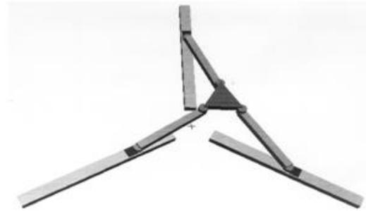
Figure 1b. A planar robot with 3-PRR configuration [11]
