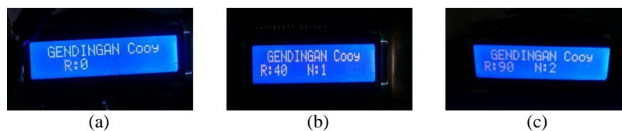
Figure 7. (a) MRE sensor display at home base position; (b) MRE sensor display at first gamelan key position; (c) MRE sensor display at second gamelan key position
