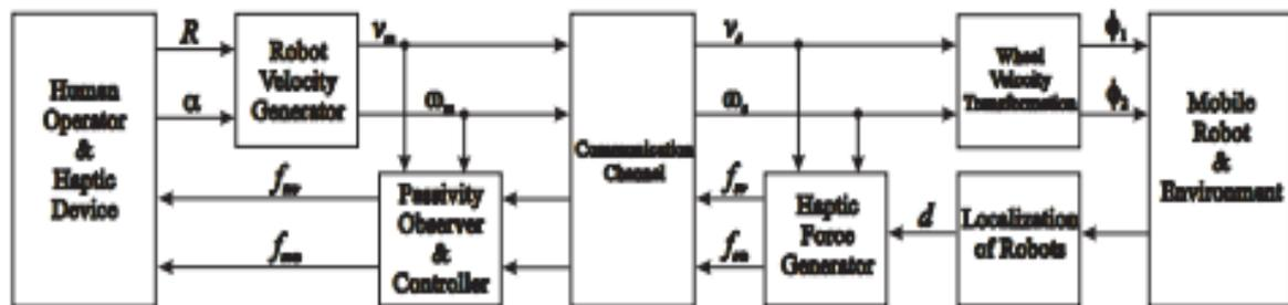
Figure 2. Items of a mobile robot teleoperation system
