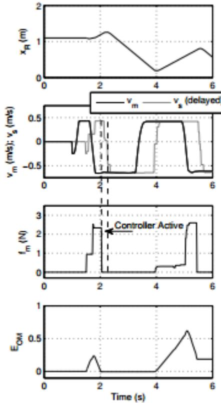
Figure 7. Behavior of the supervisor controller in the presence of large delays
