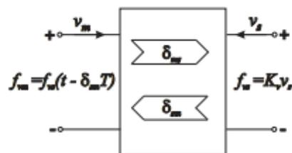
Figure 5. Communication channel as two port network
