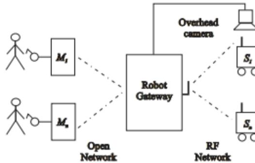
Figure 1. Block diagram of the teleoperation system
