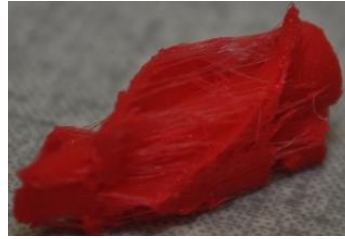
Figure 5. Outflow stator with stringing issues resolved
