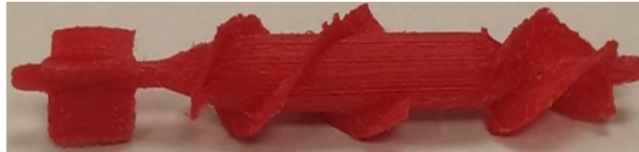
Figure 7. Full part with stringing and supports removed
