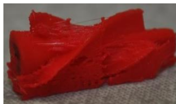
Figure 4. Outflow stator with stringing issues
