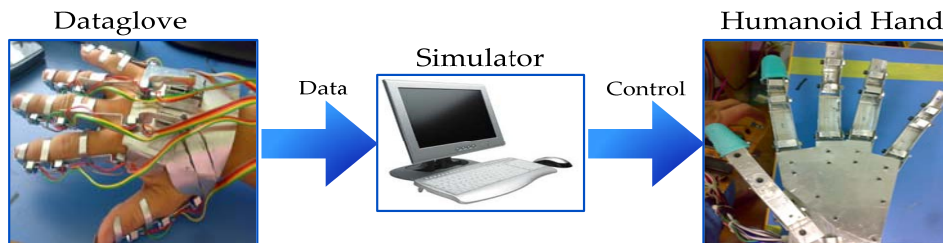
Figure 5. Control of humanoid hand using dataglove
