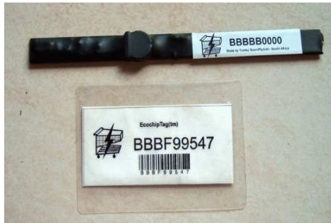
Figure 1. Stick tag & card sized transponders
