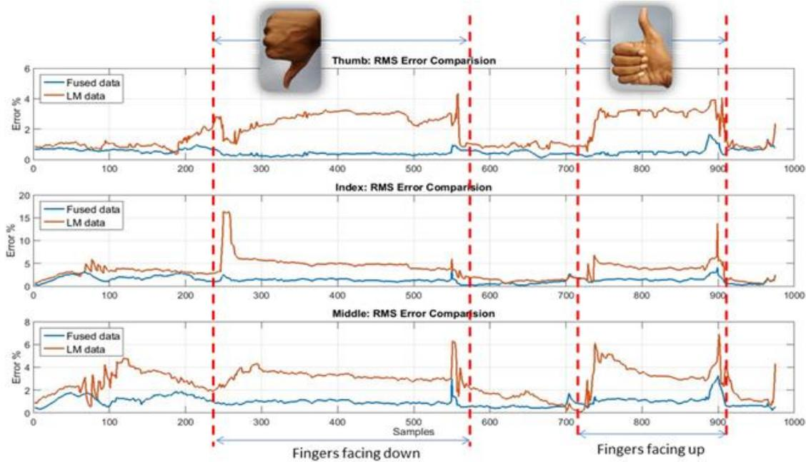
Figure 6. Comparison of RMS errors of LM alone and the proposed sensor fusion method for fixed hook grasp (OK sign)
