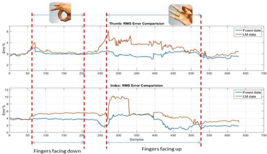
Figure 7. Comparison of RMS errors of Leap motion alone and the proposed Sensor fusion method for Tip pinch
