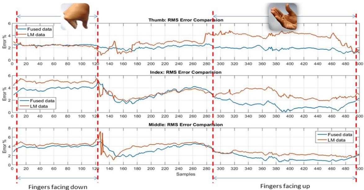
Figure 5. Comparison of RMS errors of LM alone and the proposed Sensor fusion method for Parallel extension
