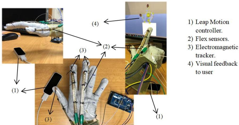
Figure 3. System components in experimental setup
