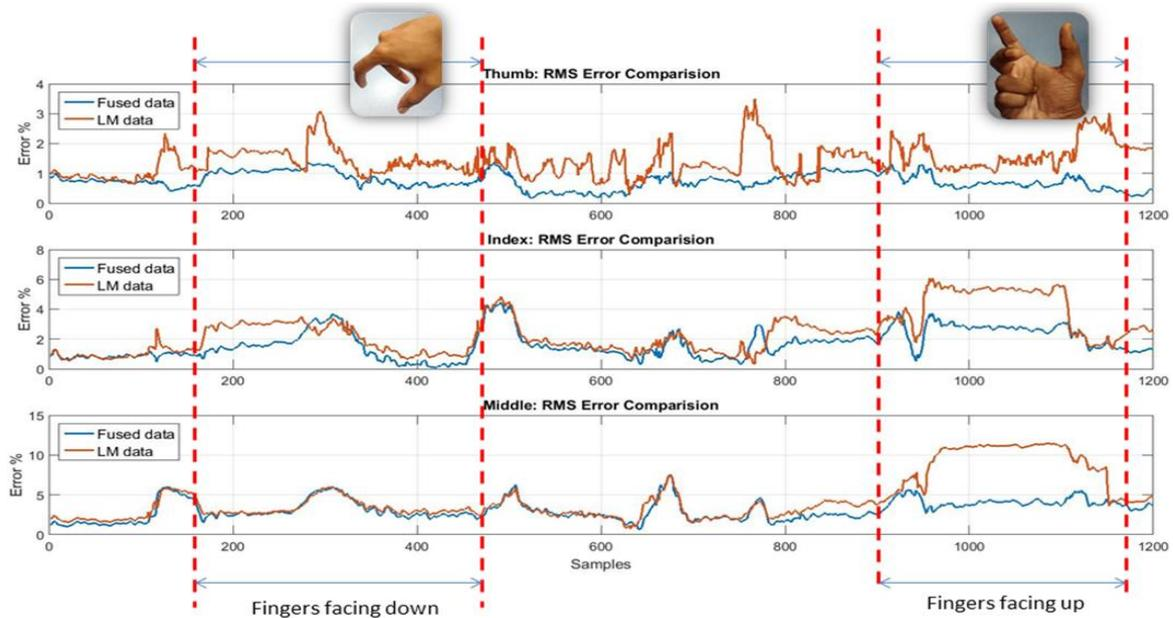
Figure 4. Comparison of RMS errors of LM alone and the proposed Sensor fusion method for 3 finger sphere formation
