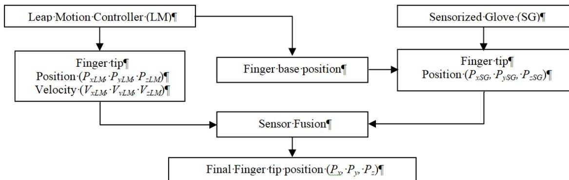
Figure 1. Overall System structure
