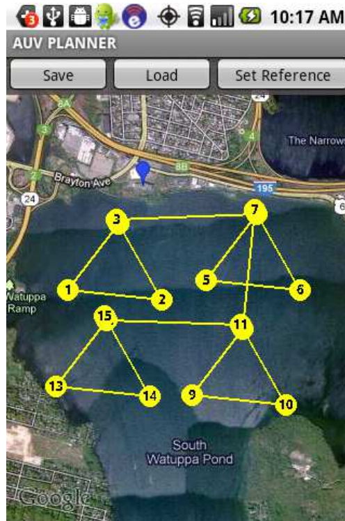
Figure 2. Using a waypoint template to insert 4 identical triangular waypoint patterns.
