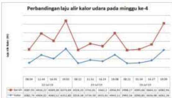
Figure 9. Comparison of heat flow rate of clean and dirty at week -4
