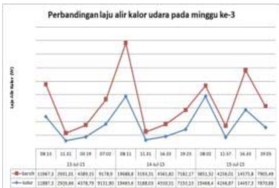
Figure 8. Comparison of heat flow rate of clean and dirty at week -3
