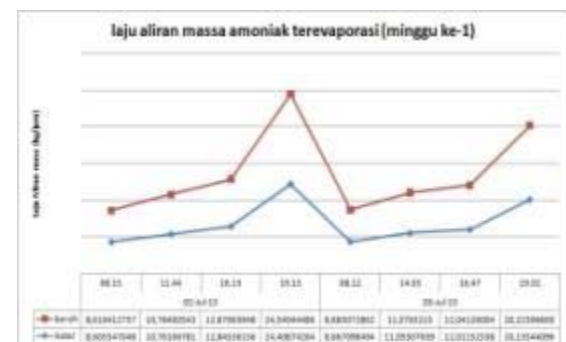
Figure 10. Comparison of the mass flow rate of the additional ammonia evaporated by week -1
