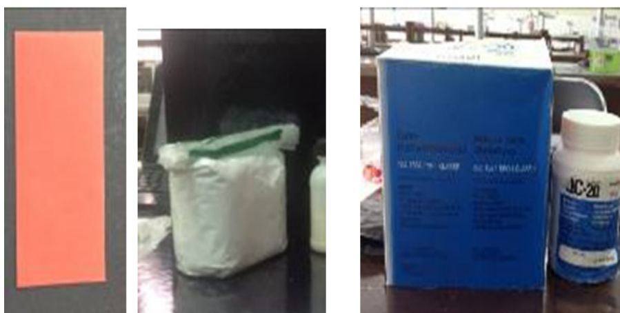
Gambar 1. (1) Baseplate wax, 2.Gips, 3. Heatcured Acrylic resin (De Trey QC-20)
