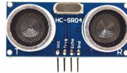
Gambar 4. Sensor Ultrasonic HC-SR04
