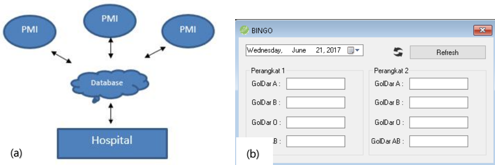
Fig 3. a) A database provides the access between IRC and hospital, so that both parties are able to share information. This database will ease the process of blood monitoring of a certain area in real time. b) The value of blood stock is displayed using Microsoft Visual Studio software.
