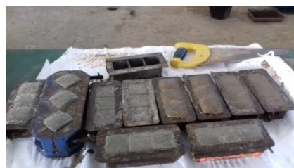
Figure 1: The result after the mixture is put into the mold and left for 24 hours.
