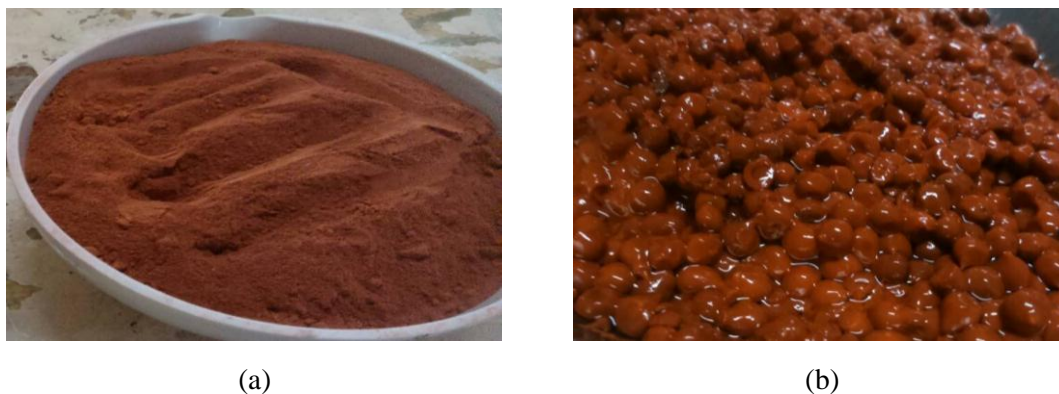
Figure 3. (a) Laterite soil from East Kotawaringin and (b) Composite Beads
