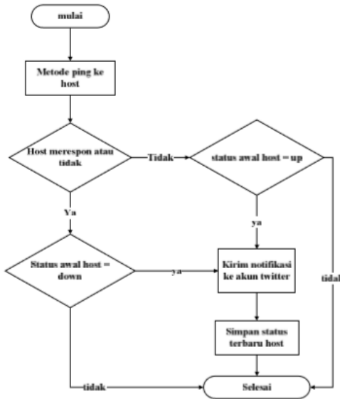
Figure 2. The ping system workflow
