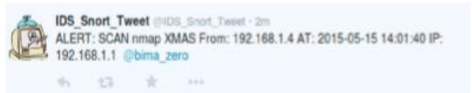
Figure 7. Notification on Twitter when the network is scanned by Nmap
