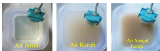
Gambar 11. Pengujian Sensor Turbidity
