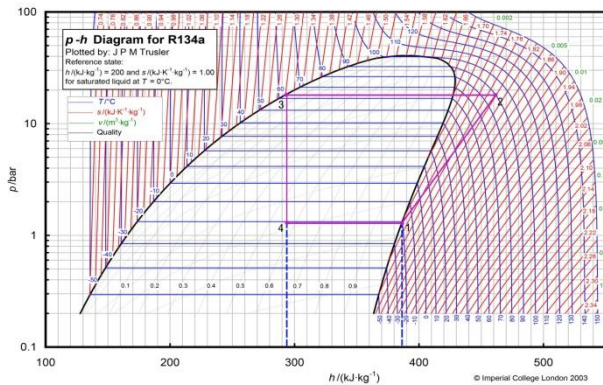
Gambar 10. Siklus p-h diagram AC mesin innova 2KD-FTV
