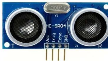
Gambar 5. Sensor ultrasonik (Ping) SR04
