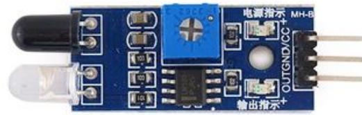
Gambar 4. Modul Sensor Jarak *Infrared* (FC-51) [4]
