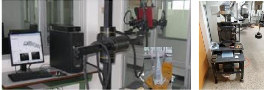
**Figure 6** Experimental setup (left) 3D scan GOM ATOS (right) ASTM G65/ G105
