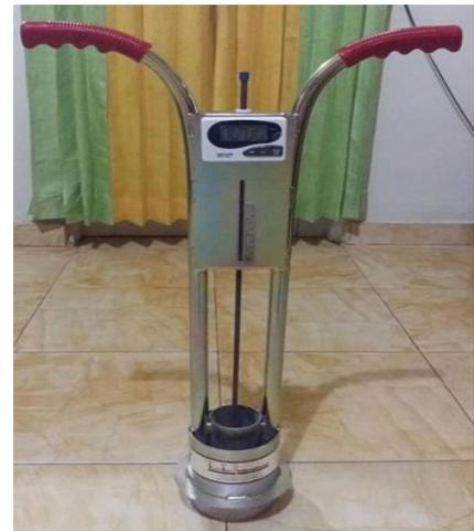
**Gambar 3.** Digital Infiltrometer
